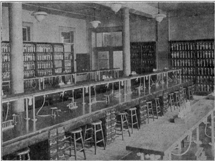
Fig. 1.—Pharmacognosy laboratory, University of Illinois School of Pharmacy. The laboratory accommodates 72 students working at one time; each student having approximately six square feet of working space. Desks are equipped with gas, water, electricity and sink, locked drawers being provided for the keeping of apparatus. The case to the right of the door contains the microscopes and the collection to the right of that includes drugs official in foreign pharmacopœias. The collection on the left wall is described under Fig. 2.
